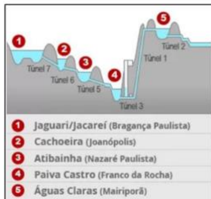
Cantareira Water Production System Schema. Source: G1
