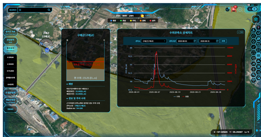
Figure 6. Real-time river water level measured on the digital twin platform.
